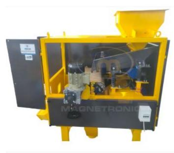
manufactured magnetic destoner is specially designed for removing mud balls and other iron impurities which can be found in wheat, dal, and other pulses where high-intensity magnetic destoner are hugely used. It is having good performance for removing mud balls for gaining 100% accuracy after passing the material on Magnetic Destoner.
